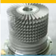
Turbo section: aluminum rotor with turbo stages designed to optimize pumping speed for light gases
